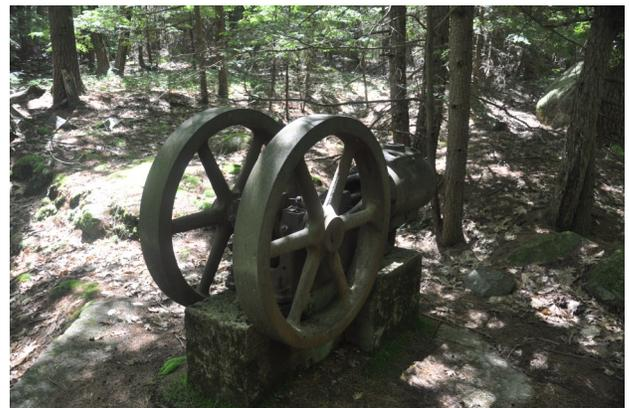
The air compressor used to drill holes in the granite
